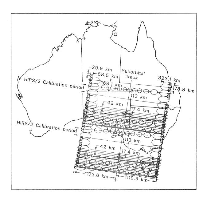
Fig. 1: Typical TOVS orbit showing the resolution of the HIRS and MSU instruments. The orbital direction is from the top right to the bottom left of the figure.
