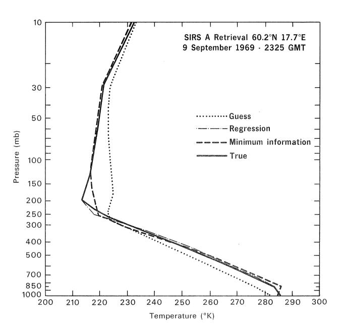
Fig. 7: Comparison between SIRS-A derived temperature profiles and a conventional RAOB (True)
