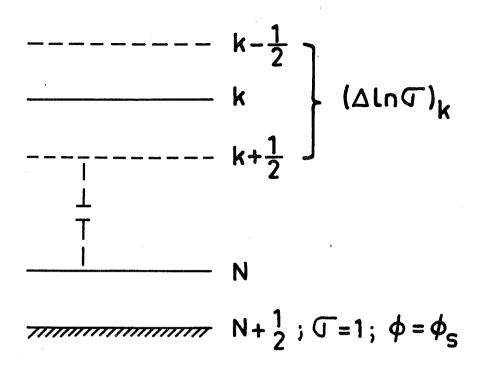
Fig. 1. Simplified display of vertical grid notations of the ECMWF models.
