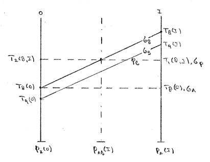
At the neighbour point the  $\zeta$ -value  $\zeta_A$  is determined by the pressure level, corresponding with  $\zeta_8$  in the central point. Next it is suppose that the temperature at this level is constant and equal to  $T_8(0)$ . Finally,  $T_1$  (8) is calculated by linear interpolation between  $\zeta_A$  and  $\zeta_9$ :
