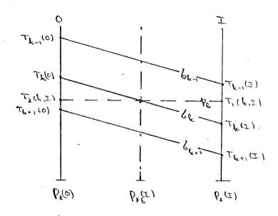
$\mathbf{T_1}$  (k,I) is obtained by simply linear interpolation between  $\mathbf{T_{k-1}}$ and T<sub>k</sub>:
