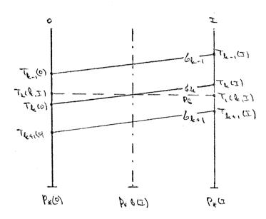
Again  $T_1(k,I)$  is obtained by linear interpolation, in this case between  $T_k$  and  $T_{k+1}$ . If  $\sigma_k$  is the lowest level, extrapolation might produce unrealistic high temperatures, therefore in this case  $T_1(k,I)$  is approximated by averaging the temperatures of central and neighbour point at the main  $\sigma$ -level:
