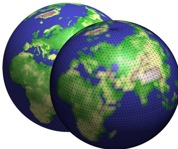
**Figure 4** Surface geopotential height field (in  $\text{m}^2 \text{s}^{-2}$ ) interpolated from an octahedral reduced Gaussian grid TCo1279 (HRES operational grid, back) to low resolution TCo31 (front). The colour palette is qualitative, for illustrative purposes only.
