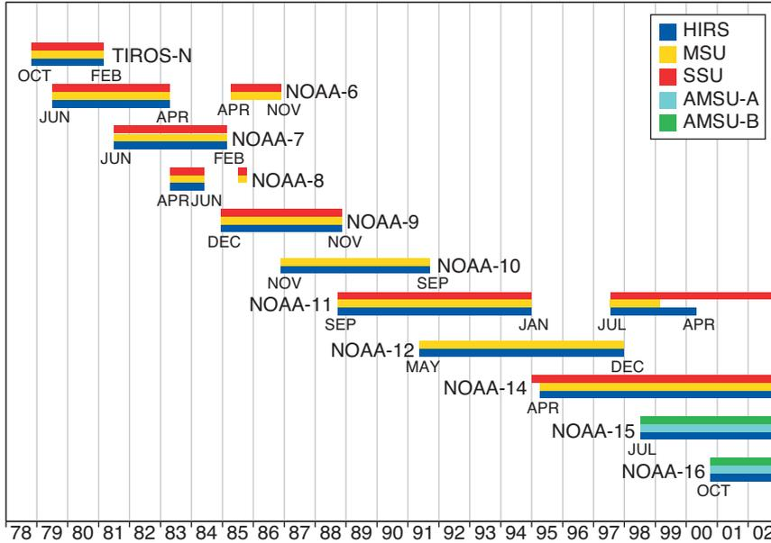
Fig. 7 Satellites with TOVS/ ATOVS instruments from 1978 onwards.
