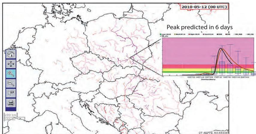
**Figure 3** EFAS forecasts from 00 UTC on 12 May 2010. All rivers which maybe affected by flooding are shaded in red and purple. Also shown is a hydrograph, which predicts a peak in 6 days. The box plots on this hydrograph represent EPS forecasts: the black line shows the ECMWF high-resolution forecast and the brown line the DWD forecast. The green area indicates the low flood warning level, the yellow the medium, the red the high and the purple the extreme flood warning level.
