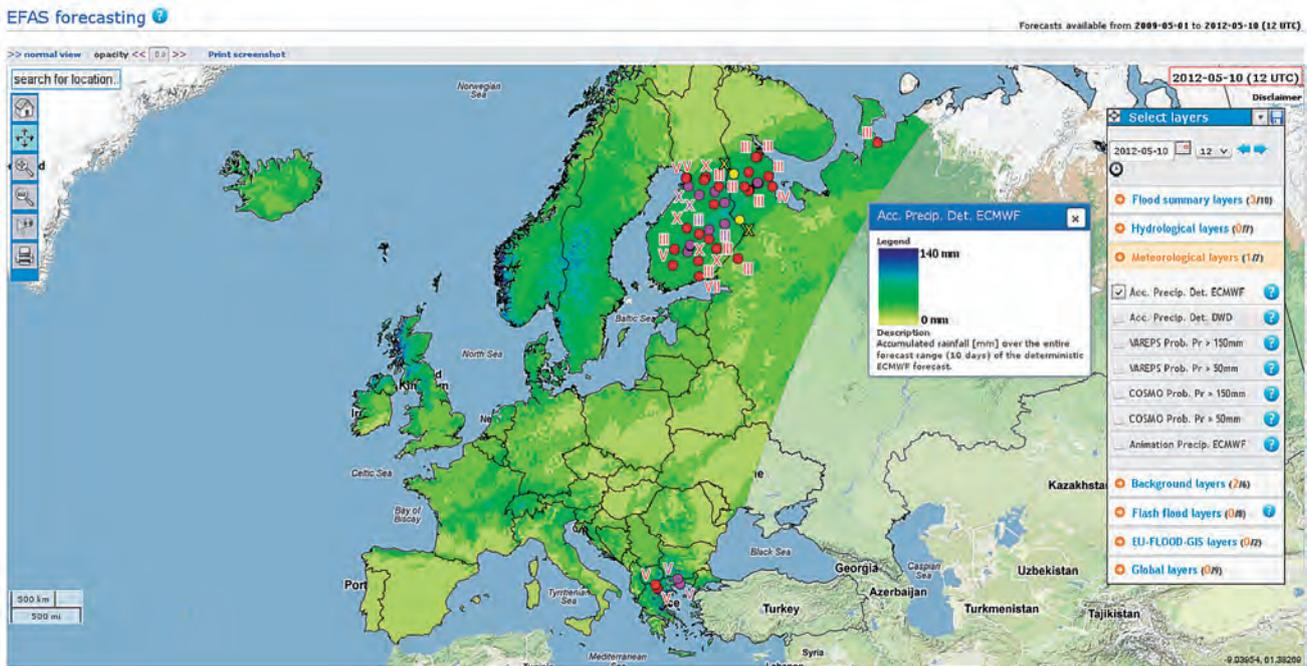
**Figure 5** Screenshot (DATE) of EFAS-IS displaying reporting points where the maximum discharge is expected within the next 5 days or more. Roman numerals denote when the maximum discharge is expected. The colours indicate the highest alert level exceeded by a certain forecast (purple being extreme and red being high).
