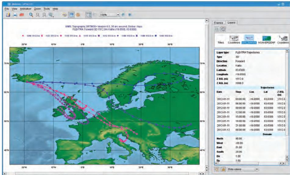
**Figure 3** Three-dimensional forward trajectories, released from the same point but at different times, visualised using an automatically-generated colour palette. The sidebar on the right-hand side of the window displays detailed statistics about the visualised data.
