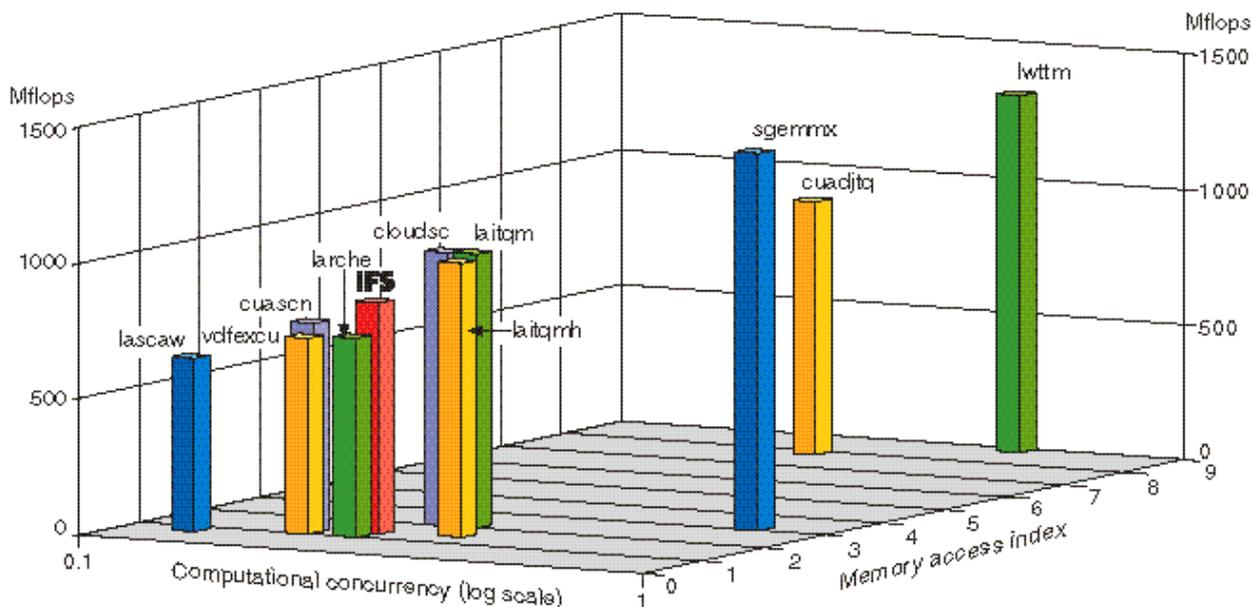
Figure 3 (below): Performance related to add/multiply overlap and the way in which memory is accessed.
