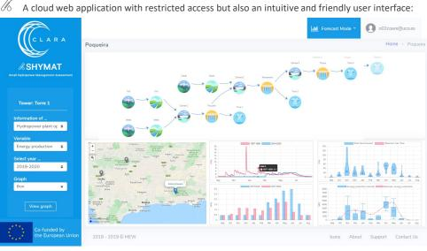
1) A geolocation map which presents the user all the hydropower systems included in SHYMAT; 2) A topological panel module which shows the elements of the RoR system (basins, rivers, load chambers, hydropower plants, and power grid), interconnected according the system operation; 3) A water availability and operation module which provides users with past, present and future information.
